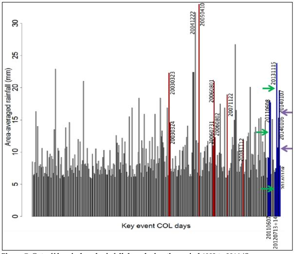
Figure 7: Cut-off low induced rainfall days during the period 1983 to 2014 (Source: RADAR 2016)
