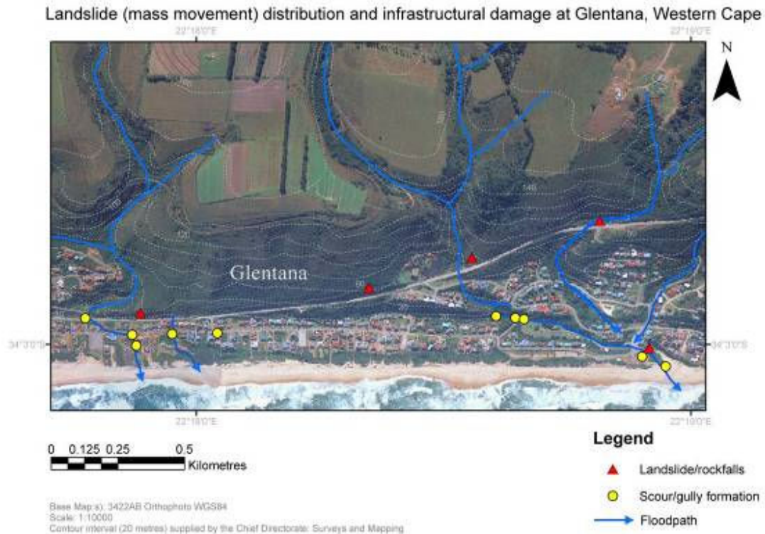
Figure 2.3.4.3.2: Landslide (mass movement) distribution and infrastructural damage at Glentana, Western Cape. A number of non-perennial streams are highlighted and represent proposed floodways of the surface run-off
